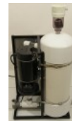
This view shows the pump and tank on the OSW-3. The vent on top of the system will remove any off gassed air and ozone for safe operation.
