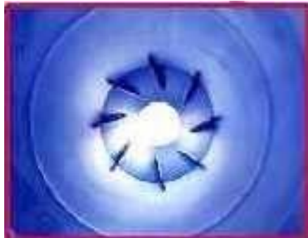
Ozone Injectors have internal mixing vanes to improve mass transfer efficiency, suction capacity & mixing capabilities.
